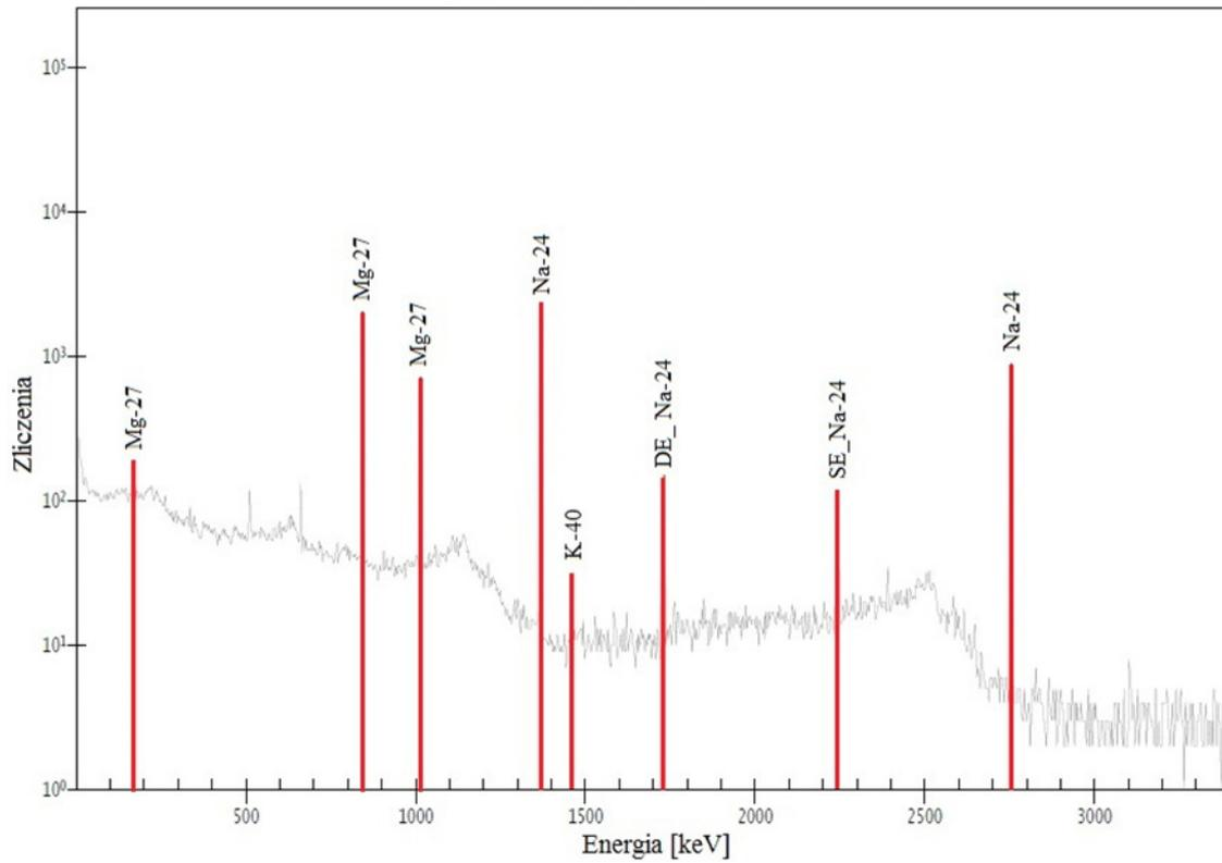
The gamma spectrum recorded for sample made from 316L(N) steel irradiated in 14 MeV neutron flux.
